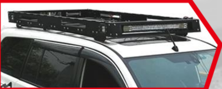
RR-SJ-001 material thickness 1.8 mm
