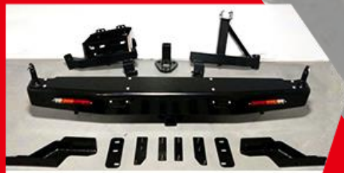
RB-TH-003 material thickness 3-5 mm weight 35 kg Package dimensions 160*30*38
