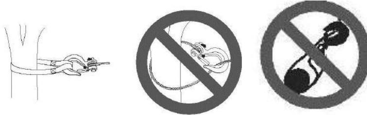
Do not wrap the wire rope around the object and hook onto the wire rope itself. This can damage the object being pulled, and kink or fray the wire rope.
